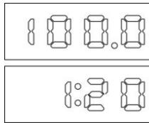
Cursor flickers in the temperature window, press or set, system will confirm new setting after 3 seconds. Set Time in a similar way as above. Pressing buttons or for 2 seconds to move cursor for quick set.
