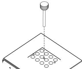
3) Lift upward the block lifter and take out block.
