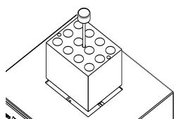
4) Place the needed block into the instrument, fix the block screws.
