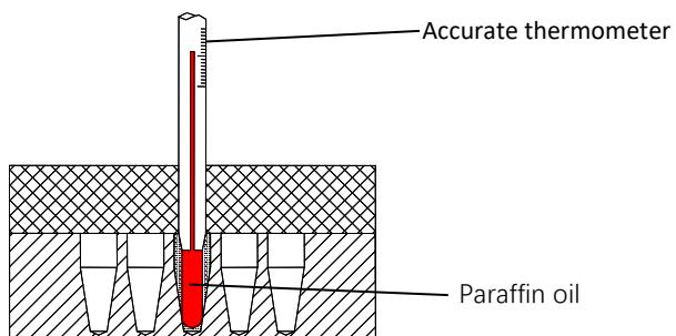
temperature ball should be absolutely immersed into the cone-shaped well). Heat insulation material is needed on the block to separate it from the circumstance. Seeing from Fig a.
