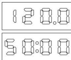
2) The dot of temperature value only stops flickering after instrument reaches target temperature. The symbol ":" of timer flickers after the temperature reaches demanded value and timer starts to count down.
