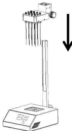
**Note: Make sure the carriage is tightened well on the column before use.**
