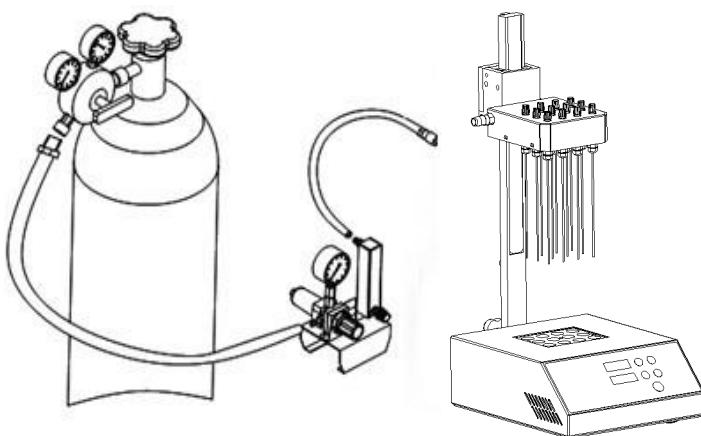
Connect the airflow valve with gas distributor by a shorter (1.5M) gas pipe, connect the airflow valve with the gas generator by a longer (3.0 M) gas pipe.
