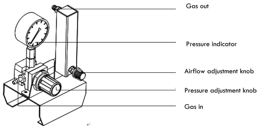
Pull out the airflow adjustment knob, turn it clockwise direction to increase airflow, on the contrary, turn it anticlockwise. Push the knob again to lock it.
